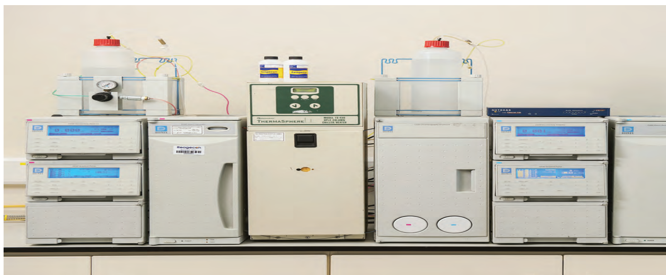
Reagecon's Dionex Ion Chromatograph with CD20 conductivity Detector, EG40 Eluent Generator, LC20 Chromatography Enclosure, GP40 Gradient Pump, AS50 Autosampler & Phenomenex TS-430 HPLC Column
