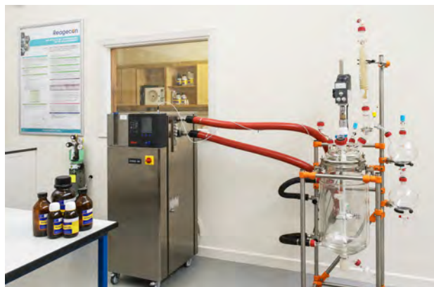
One of a suite of temperature controlled distillation and reflux apparatus photographed in our purification, synthesis and raw material characterisation laboratory.
